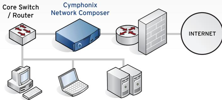
Network Composer is a secure Web gateway appliance that sits between your corporate firewall and network switches. It comes fully-loaded with everything you need to reveal, optimize and protect your Internet connection. It features a convenient and powerful Web-based management console and receives frequent automatic updates to protect your organization from emerging threats.
